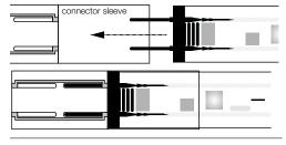
4. The end cap must be glued on to the end of the strip. Allow the alue to dry for 15 minutes.
