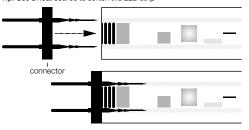
3. Apply glue to the end of the hose over a length of 2 cm and then insert it into the connector sleeve. Let the glue dry for 15 minutes
